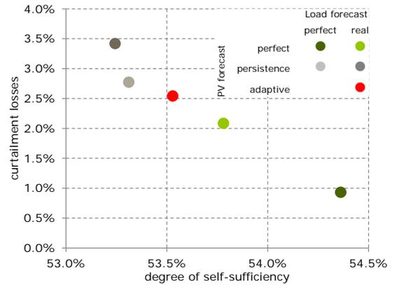
**Figure 8:** Comparison of the operational results of the adaptive forecast approach.
