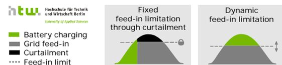
**Figure 1:** Schematic representation of different operation strategies
