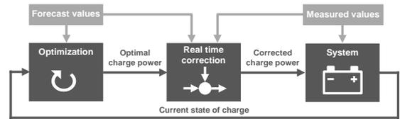
**Figure 2:** Control scheme of the forecast-based operation strategies .
