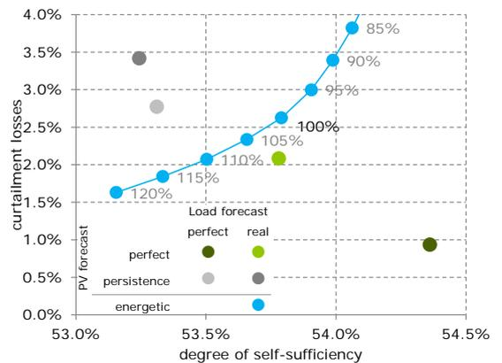
**Figure 5:** Influence of systematic forecast errors on energy PV forecasts for dynamic feed-in limitation.
